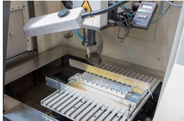
Figure 5: Drilling in the laser system
